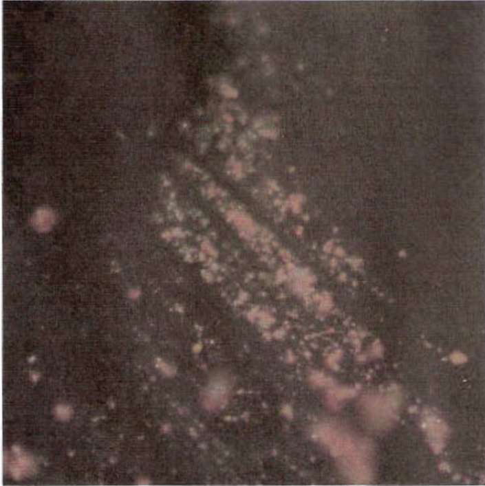
Birdwood Sample 1. Red wash pigments Crossed Polars (darkfield) 400X
